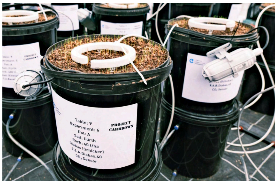
Greenhouse lysimeters with CO 2 sensors: The gray pill-shaped tubes contain controller, antenna and battery, the cable leads to the sensor buried at x cm in the soil.
